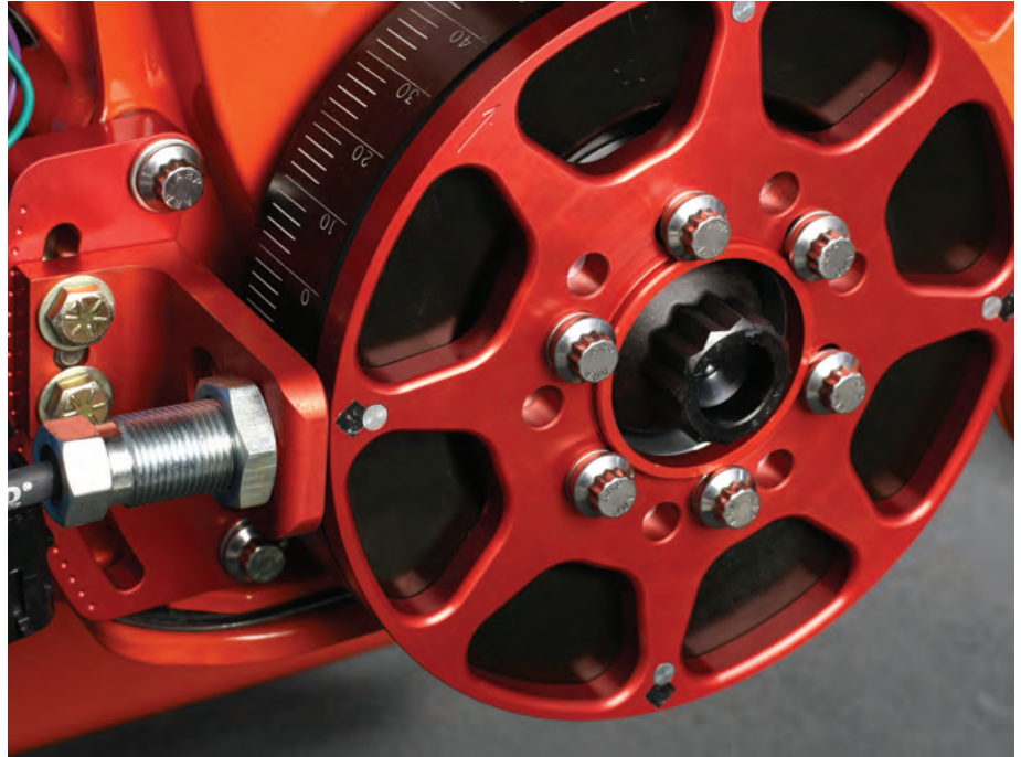
Anodizing protects the alloy surface from oxidation and corrosion. The color dye is added simply for the sake of appearance.
