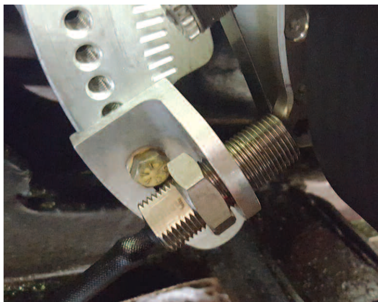
In order to get the crank position, Holley uses this external crank sensor, which must be at a set distance from the balancer that you measure with a feeler gauge.
