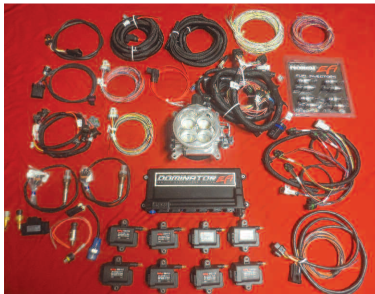
This is the full complement of Holley EFI components used for the swap including the Dominator ECU, ignition coils, 160 lb/hr injectors, throttle body, NTK wideband O2 sensor, and wiring harness.
