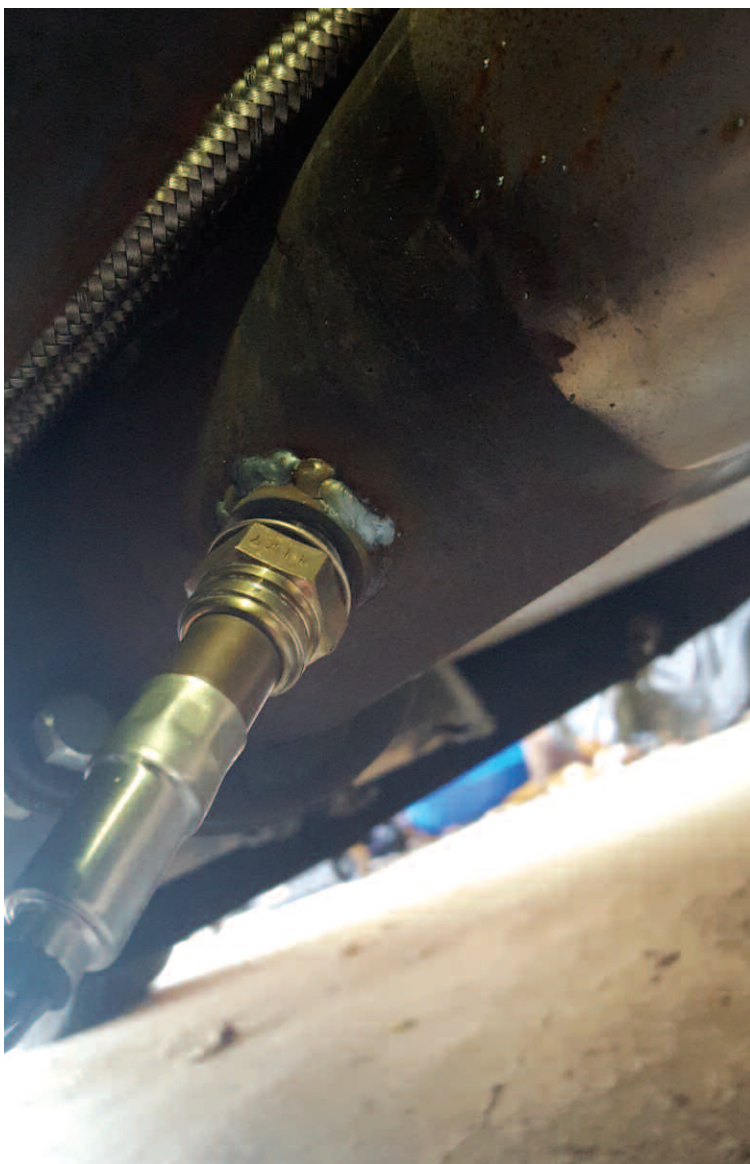
If you don't already have one, you need to weld a bung into the exhaust for the wideband O2 sensor. The Holley EFI adjusts the fueling based upon the wideband O2 sensor readings, and can also data log air/fuel ratio along with many other inputs.
