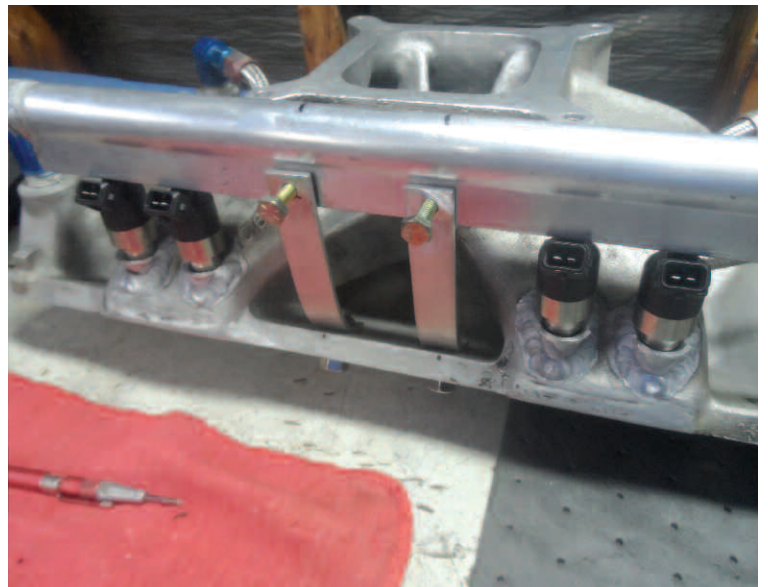
The Holley 160 lb/hr injectors were put into the rails one last time to mock up the supports for the fuel rails.
