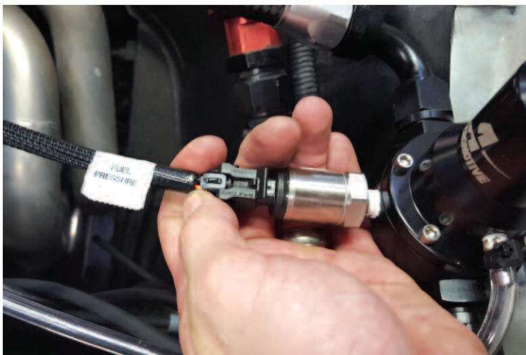
The fuel pressure sensor and harness plug into the regulator, which will be one of many data points for the Holley EFI Dominator. There are all sorts of safety features in the software that can protect the engine such as a fuel pressure drop that would cause the engine to go lean.
