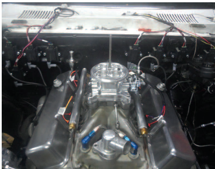
Redline chose to mount the Holley ignition coils on the firewall. New plug wires were cut to fit. By switching from a single coil and distributor, much more spark energy is available.
