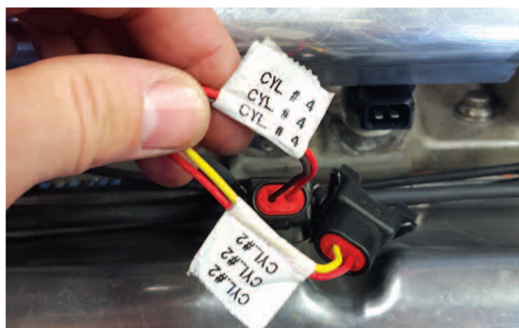
Holley clearly labels the wiring harness to avoid any issues. These simply plug into the injectors.
