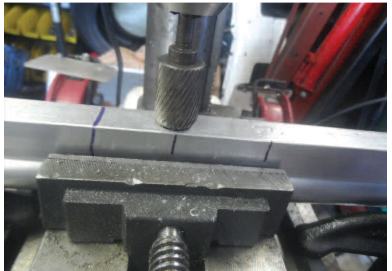
New fuel rails were fabricated using pre-made blanks. Once lined up to the injectors in the manifold, the blanks were marked, drilled and machined. A lip is needed for the O-ring, which seals the injector to the rail.
