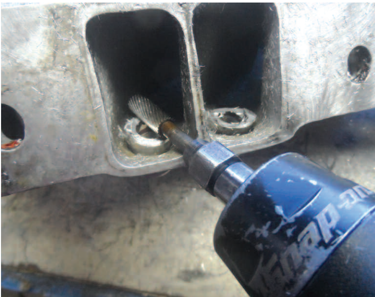
The extra material was then ground down and polished smooth so as not to obstruct the intake path.
