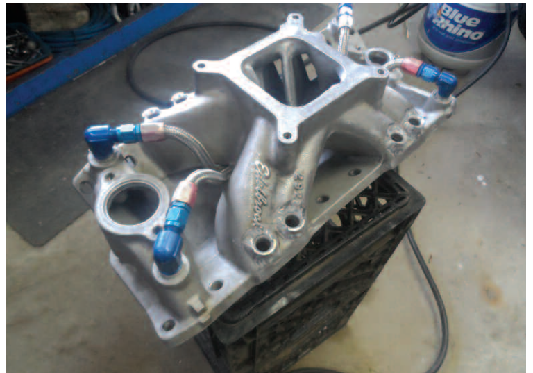
By reusing the existing intake manifold on the blown 434ci small-block, the owner was able to save a few dollars and keep our testing consistent.
