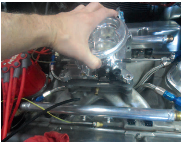
The Holley 4-barrel throttle body is a simple swap for a carb atop the intake manifold—even with the blower hat.
