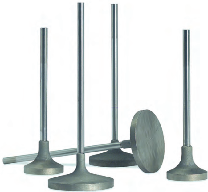
A sample of titanium valves in blank form. Stems have been machined to near-final diameter and the heads are rough formed, prior to CNC machining. (Courtesy of Xcelodyne)
