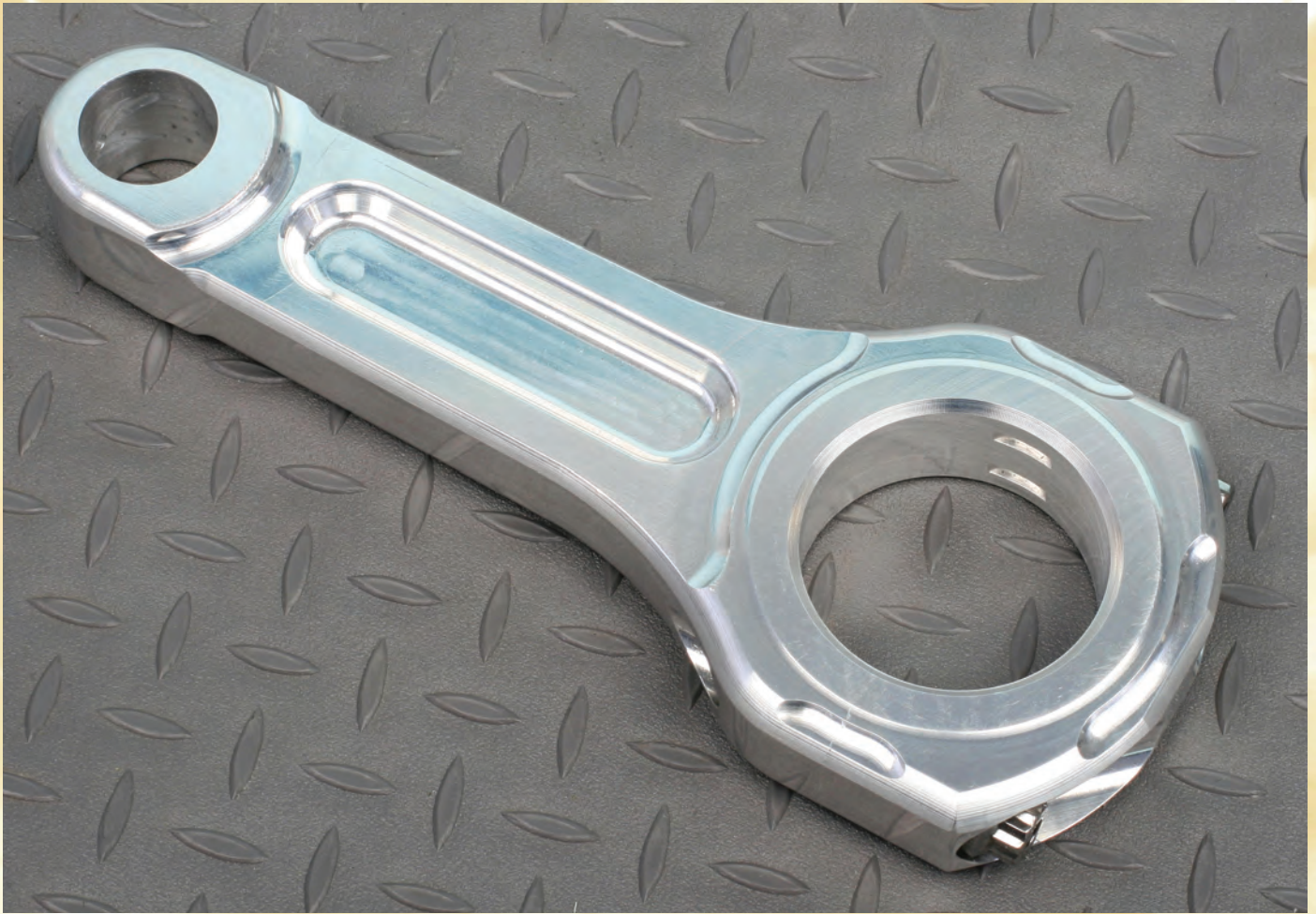
Aluminum connecting rods, although made of high-density aluminum forgings or cut from billet stock, are beefier and command more room. Extra attention to clearances between the rod big end and the block and camshaft is critical.
