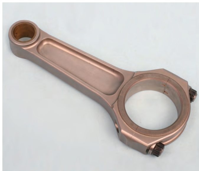
I-beam rods feature smooth beam sides and face recesses. I-beam rods are typically lighter than H-beam designs. Depending on material, length and application, forged steel I-beam rods are generally viable for 500-700 HP applications.
