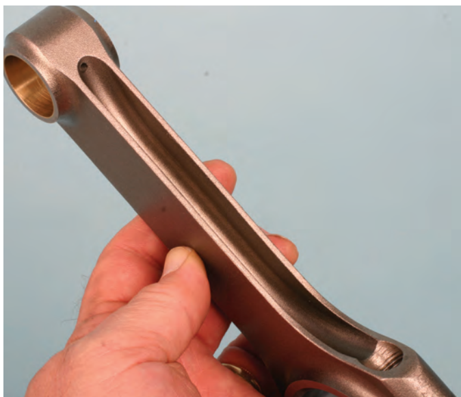
The deep groove on the beam sides of an H-beam rod reduce weight and provide extra rigidity for higher horsepower and torque and higher-RPM applications, as compared to I-beam rods.
