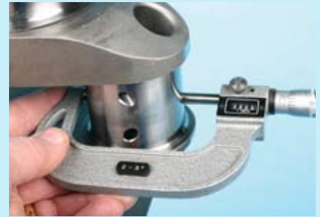
Check each rod journal not only for diameter, but for centerline (stroke) distance relative to the main centerline.
