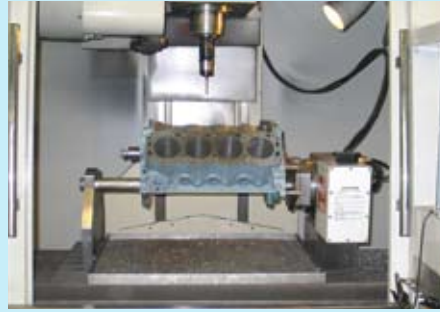
Here a block is mounted in a CNC machine, ready for measuring and machining.
