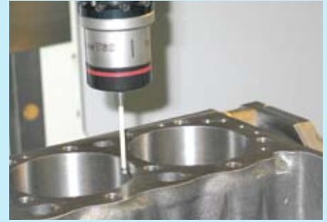
CNC probing records existing cylinder bore location. This derived dimension can then be compared to design data, instructing the machine to then bore to correct centerline and angle if needed.
