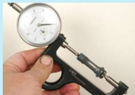
Measure free-length of each rod bolt as reference, and keep them organized.
