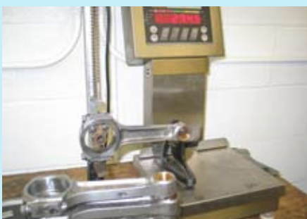
Weigh and weight-match all components. Don't assume that all rods, pistons, etc. will be identical.
