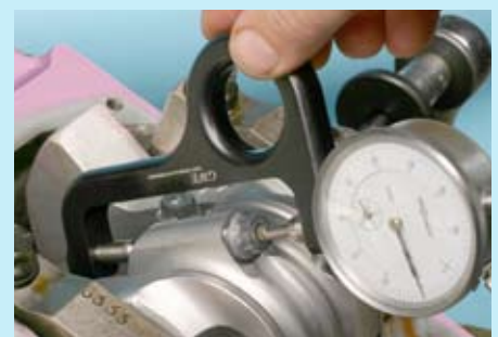
If tightening via the stretch method, measure and record each rod bolt's installed length.
