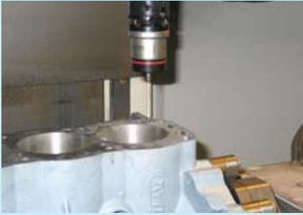
Here the CNC probe measures (and records) existing deck surface height and angles.
