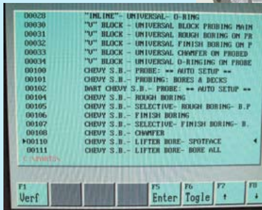
Today's engine-builder-specific CNC machines offer ready-made programs for machining specific make/model blocks for achieving precise dimensional control.
