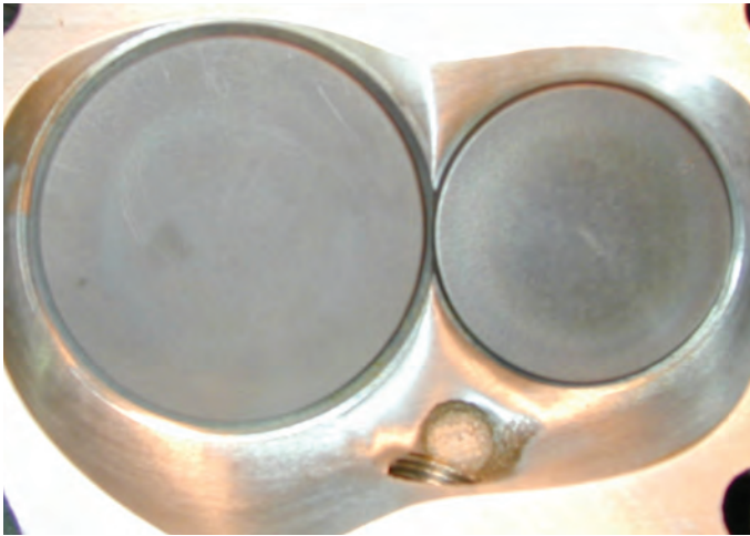
Figure 6 & 7. The combustion chamber on the intake side is of a laid back design that probably enhances the airflow path from decreasing the shrouding of the intake valve. The only way to be sure is to measure the results on a flow bench.
