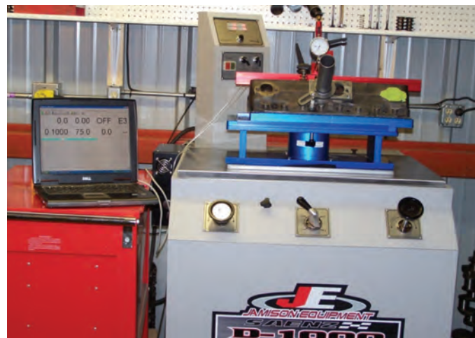
Figure 4. Super Stock cylinder heads have specific rules to follow and ports can be reshaped but they must maintain mandated sizes. All exhaust testing should use a pipe to get correct flow numbers. This 1000cfm flow bench provides accurate numbers for developing components and keeps quality control on the heads at a high level. (Photo courtesy of Stu Zylstra.)
