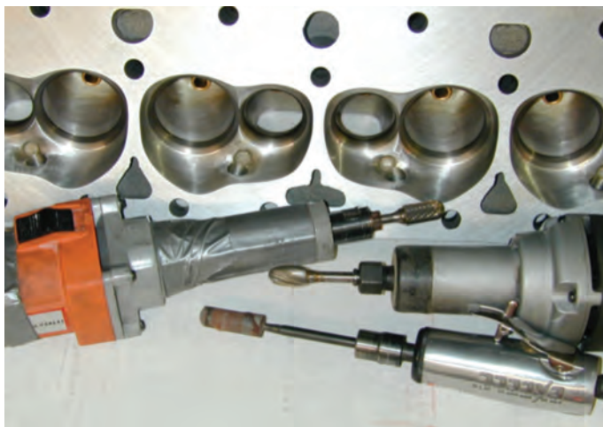
Figure 3. A grinder is about the last thing that should be picked up when planning on improving the airflow of cylinder heads. First you have to know what needs to be done in order to be effective and random grinding may not be the correct answer. Often what looks good might not flow well.
